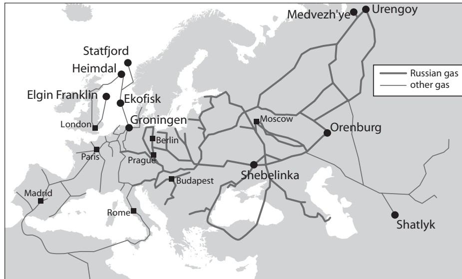
FIGURE 5 The world's longest (and largest-diameter) natural gas pipelines transport fuel from western Siberia to western Europe. The next stages of Russia's global energy importance will include natural gas and crude oil pipelines for exports to Japan and China and eventually also massive liquefied natural gas exports to the United States.
